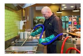
We pump the oil from the fryer into the filtration machine.
